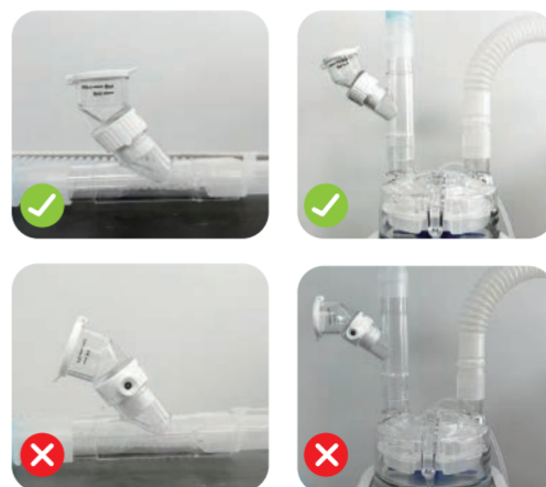
Fig. connection of a mesh nebulizer and Y-piece in a breathing circuit
